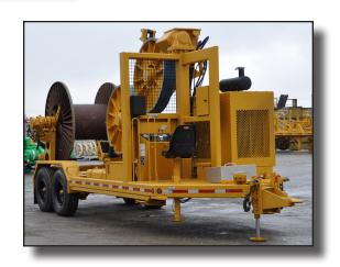
The SPT40-1H/SL is a trailer mounted, self-loading puller-tensioner suitable for new construction and reconductoring construction. This unit is capable of pulling or tensioning single conductor.
